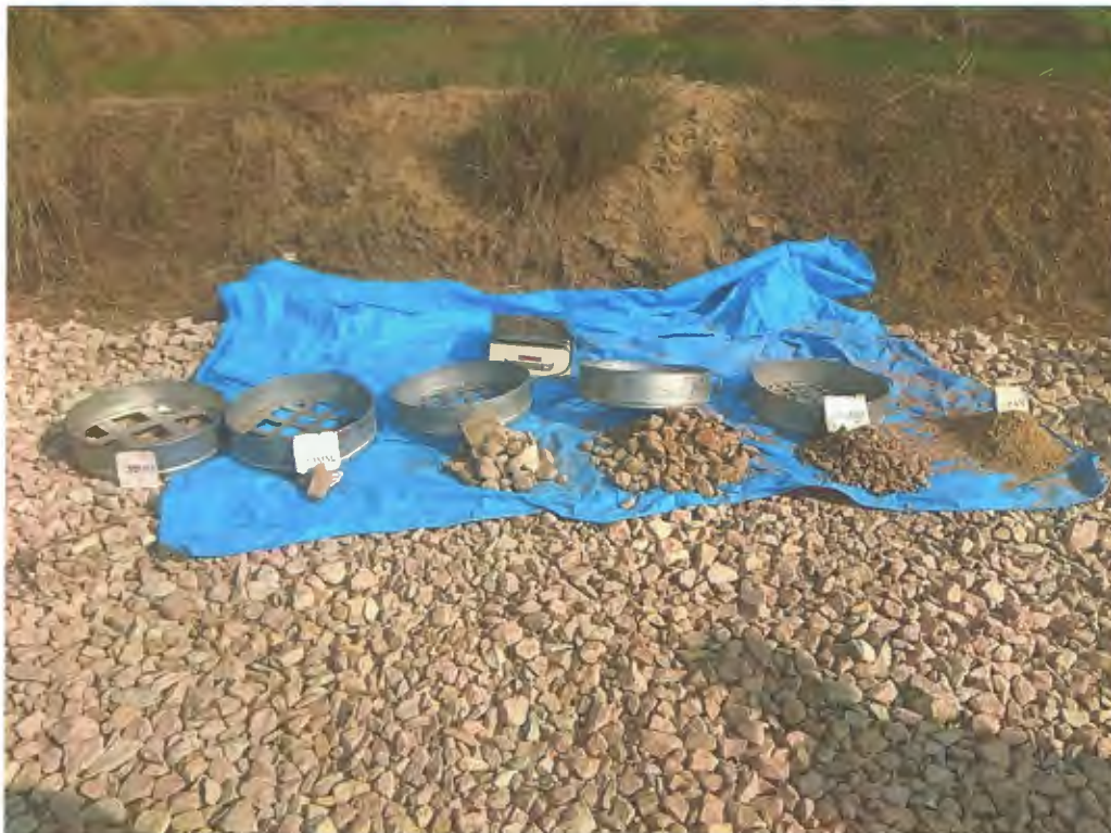
Gradation test of W.B.M. Gr II at CH 1.90 K.M
