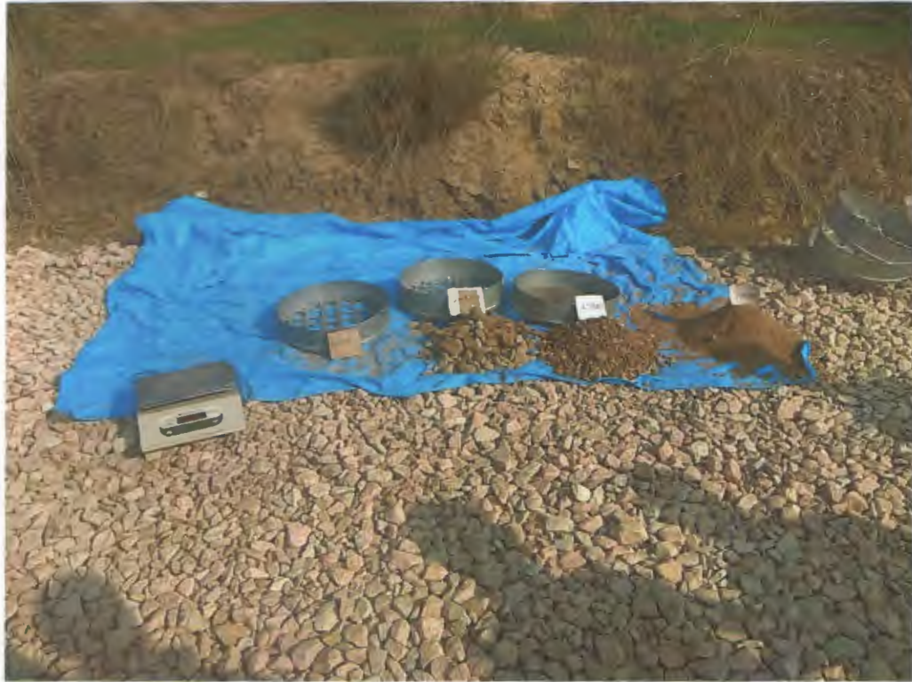
Gradation test of G.S.B. at CH 1.90 K.M
