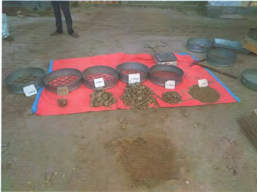
Gradation test of WBM Gr III at CH- 0.750 K.M.
